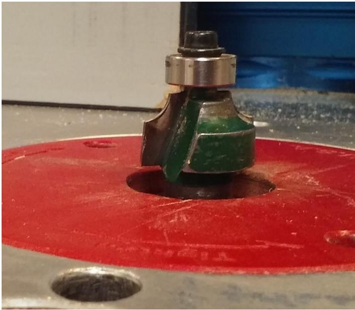
Round over the edges. Use a round over bit with a small radius on a test board. Adjust the vertical setting to get a nice cut.
